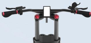
Check the instrument screws are tightened
