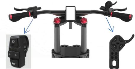
Set the use and strength of the electronic brake among the detailed functions of the instrument panel before driving. When the brake lever works, the electronic brake works together to increase the braking force.
